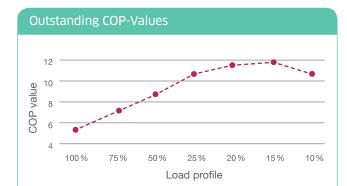
Data for the QUANTUM X060-P2C-LL chiller used at the Bamberg Concert and Congress Hall. Energy efficiency, outstanding part load efficiency and variable speed regulation lead to very good COP values.
