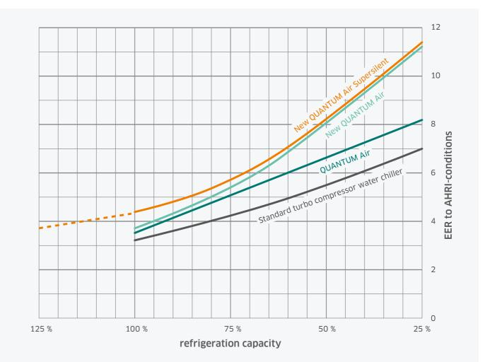
Standard turbo compressor water chiller **QUANTUM Air New OUANTUM Air New QUANTUM Air Supersilent**
