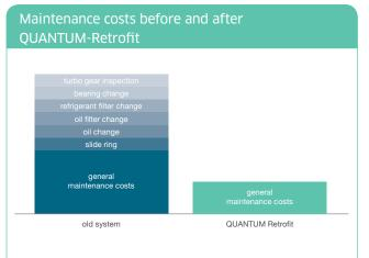
50 % less generating costs (right). Data based on a four-month study of an actual system (cold water 13/7 °C, cool water 28/33 °C).
